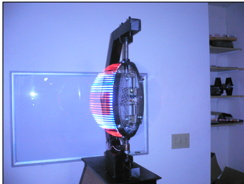
Figure 1: Persistence of vision demonstrated on SWORD.
